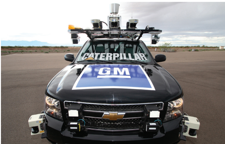
Technology touchstone: The forest of sensors on Carnegie Mellon's 2007 DARPA Challenge-winning "Boss" shows the progress made in autonomous systems during the last decade.
